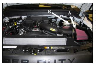
11. A) Install the Airaid Premium Filter to the mounting flange inside the quick fit assembly. B) Complete the installation by attaching the Weather Strip to the top of the panels as shown.
