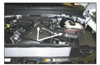
1. Disconnect the negative battery cable! Loosen the two intake clamps, unclip the coolant line, and remove the Factory intake tube.
