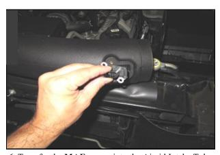
6. Transfer the MAF sensor into the Airaid Intake Tube and secure using two 8-32 x 1/2" button head screws. Do Not Use The Factory Torx Head Screws
