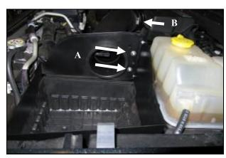
**8. A.)** Mount the Intake Tube to the Rear Panel using the two 1/4-20 Button Head Bolts and 1/4" Flat
